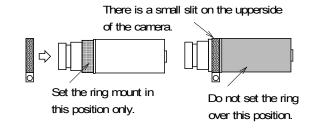
Fix the mount by passing the ring over the lens of the camera, and then attach the thread and nut.
